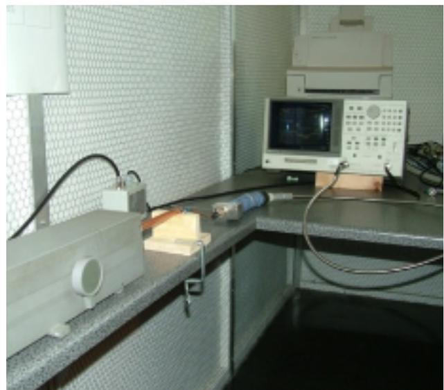
Figure 1\_Measurement of screening effectiveness using the clamp method.
